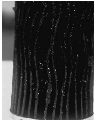
Figure 5a Example of fuel filter fouled with biomass accumulation; whole filter.
