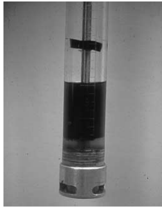
Figure 9 Typical grab sample from fuel:water interface within a diesel fuel storage tank.
